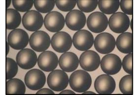
Compared to a Type I strong base anion resin, a Type II resin will yield greater operating capacity due to more complete regeneration. It is best-suited to treat water in which silica and carbon dioxide do not exceed 30% of the total anions and the service and caustic regeneration temperature does not consistently exceed 35°C (95°F).
