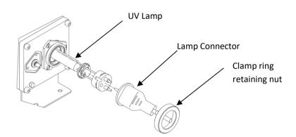
The installation of the updated Wafer<sup>™</sup> System lamps is orientation sensitive. The points of the triangular lamp cap must line up with the gaps between the internal tabs on the clamp ring, and the lamp should be left with the return rod facing down. See image below for details:
