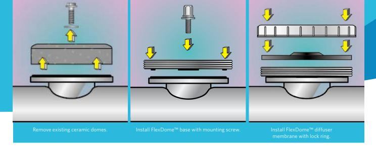
Installation is as simple as 1, 2, 3 — entire removal and installation takes less than two minutes per dome!
