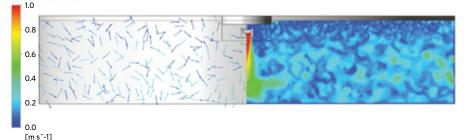
A 3HP Aqua-Lator<sup>®</sup> Direct Drive Mixer installed in a 45 ft. diameter. by 9 ft. deep tank shows that 0.5 m/s are prevalent throughout the tank, far exceeding the 0.2 m/s velocity typically recommended to keep activated sludge in suspension.
