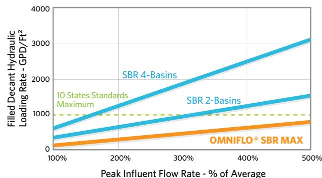
Conventional SBRs suffer from excessive influent velocity during storms. The OMNIFLO MAX fixes this issue by reducing hydraulic loading rate to as little as 17% of conventional SBR systems.
