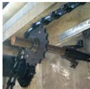
**Driven:** Non-metallic and split construction for easy installation. Dished to accommodate wall bearings and to avoid contact with flights. Replaceable or integral teeth are available.
