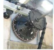
**Materials:** Teeth in polyurethane or cast nylon. Bodies in polyurethane, cast nylon or cast iron.
