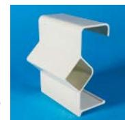
**Extensions:** Envirex flights can be provided with an integral face extension to permit more effective movement of lighter secondary or alum sludge, which can flow over shorter flights. It also provides added stiffness and strength for challenging applications. Sigma Plus extensions are available in 3 inch (76 mm) and 7 inch (178 mm) heights, and the Diamond is available with a 4.5 inch (114 mm) extension.
