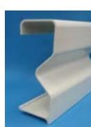
**Sigma Plus Flights:** This flight is an improvement over conventional channel flights due to its transverse concave indentation. With 60% greater structural support compared to a channel flight, it can be installed in collectors up to 25 feet (7.6 m) wide.
