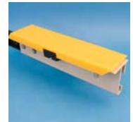
**J-Track:** Named for the unique shape of the main fiberglass structural member, this special configuration eliminates twisting and bowing for track support spacing greater than 20 ft (3 m). A UHMW PE wear strip slides on top of the J, eliminating the need for mounting hardware, maximizing the effective wearing thickness.
