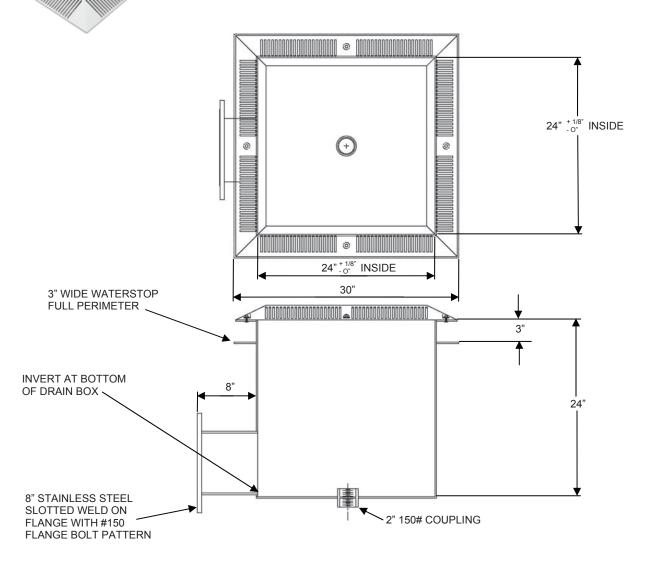
ANSI/APSP/ICC-16 VGBA 2017 & NSF 50 Certified WALL FLOW RATE: 1120 G.P.M. FLOOR FLOW RATE: 1432 G.P.M. LIFE: 15 YEARS – SUBMERGED OUTLET AEGIS by NEPTUNE - BENSON, INC.
