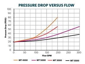
$<sup>^*</sup>$ These pressure drops are from the inlet of the trailer to the outlet connection. The MT 5000 has two trains @ 300 gpm each.
