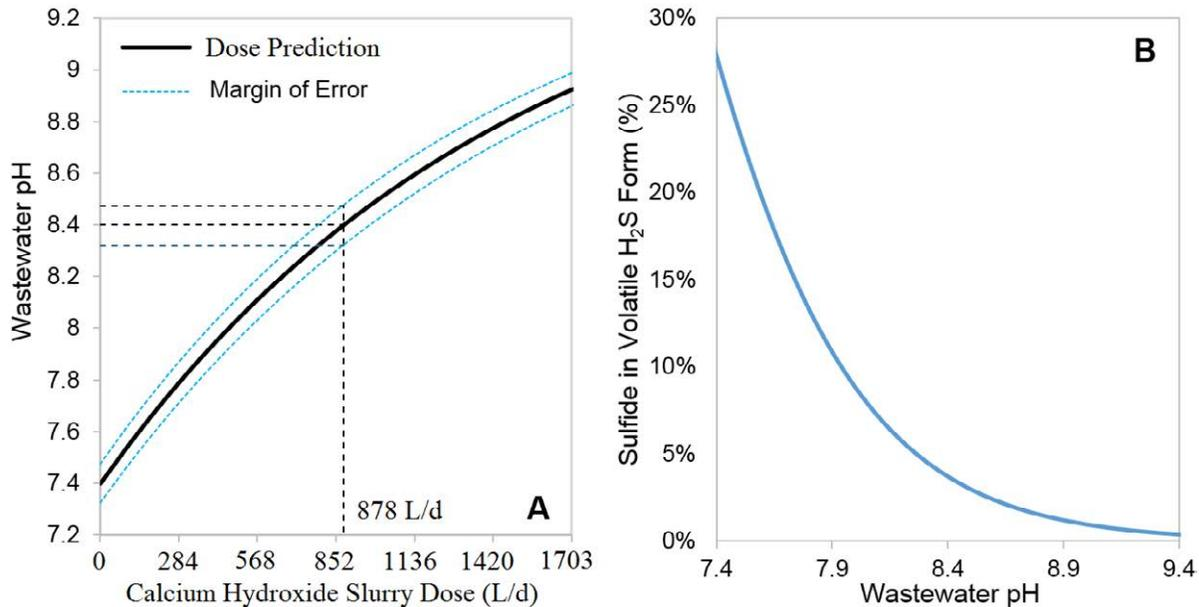
**Figure 2 – Calcium Hydroxide Slurry Dose A) Dose Predictions B) pH Sulfide Relationship**
