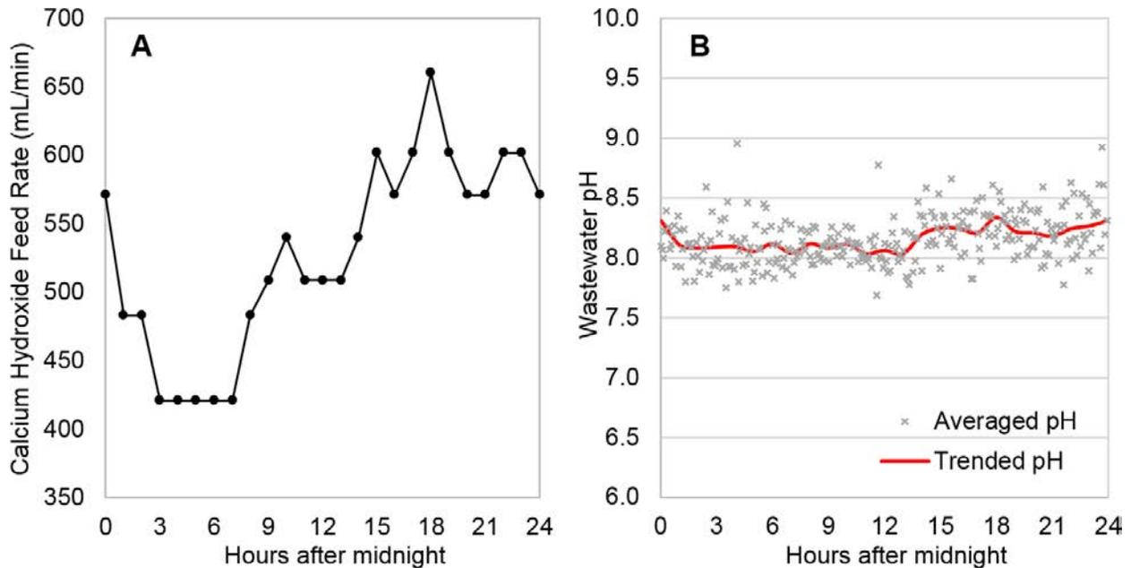
**Figure 4 – Siesta Key WWTP Optimized Configuration A) Daily Dose Curve B) Treated Wastewater pH**
